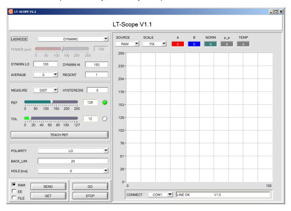
In order to avoid data transfer problems through the serial interface it is recommendable to change to the STOP mode (press the STOP button) before activating function keys and sliders.
